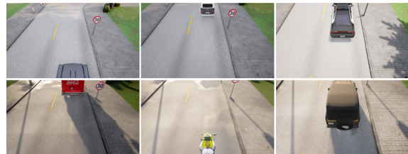
Figure 2: Overview of the different datasets. Upper row 4m camera height. Lower row 3m camera height. The columns show an 45°, 50° and 60° camera pitch from left to right.
