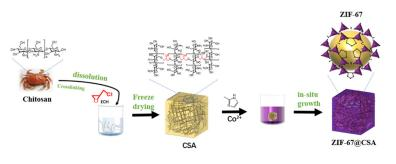
Figure 1: Schematic fabrication process of ZIF-67@CSA.
