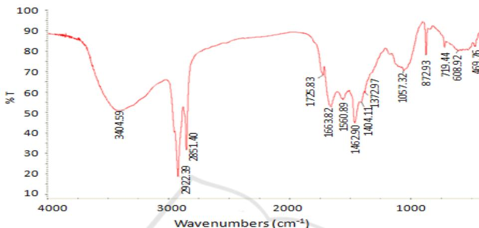
**Figure 4.** IR of retention matter on membrane after filtering sewage.
