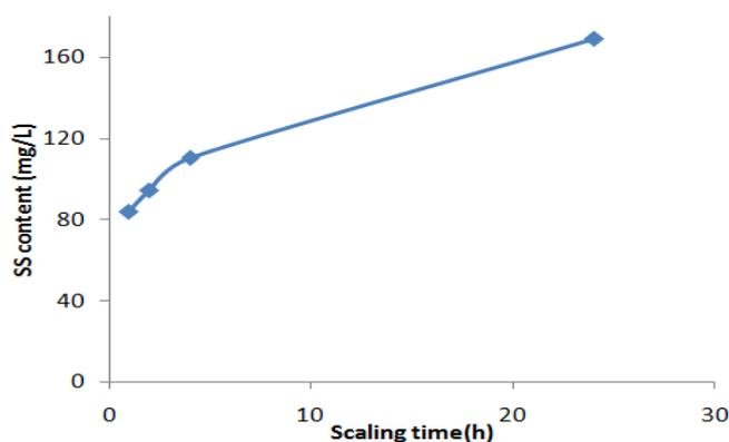
**Figure 6.**Scaling and suspended solids (SS) content variation(45 °C) for ASP flooding sewage after membrane filtration
