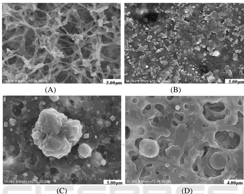
**Figure 5.** SEM images of the blank membrane (A); Membrane after filtering sewage(B); Membrane after filtering sewage and solvent extraction(C); Membrane after filtering sewage, solvent extraction and removing surface layer(D).
