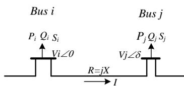
Figure 5: Representation of two bus power system.
