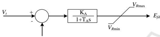
Figure 1: Exciter diagram block.
