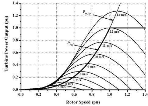
Figure 4: Characteristics of wind turbine and MPPT Curve.
