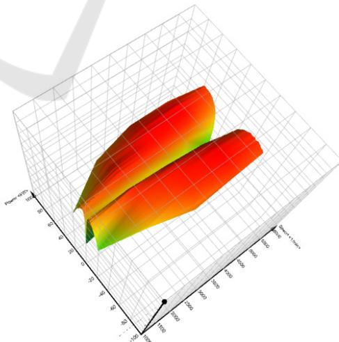
Figure 10: Efficiency map of the generator
