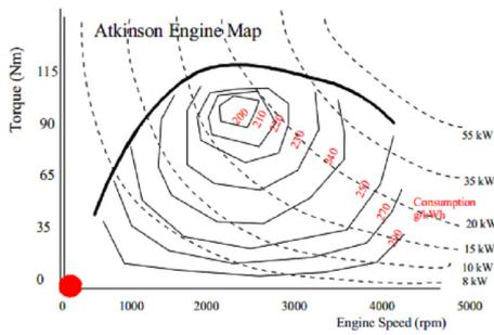
Figure1: Map of the typical Atkinson cycle engine
