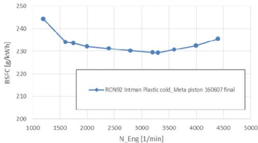
Figure11: Fuel consumption curve of the engine
