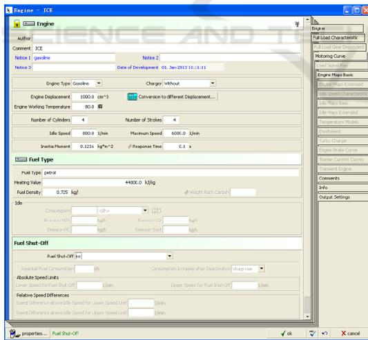
Figure 2: Input interface of basic parameters of the engine module
