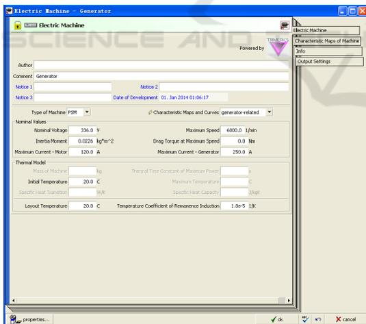
Figure 7: Input interface of the generator parameters
