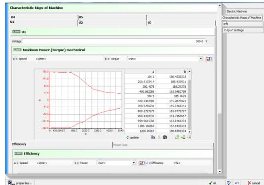
Figure 8: External characteristics of the motor
